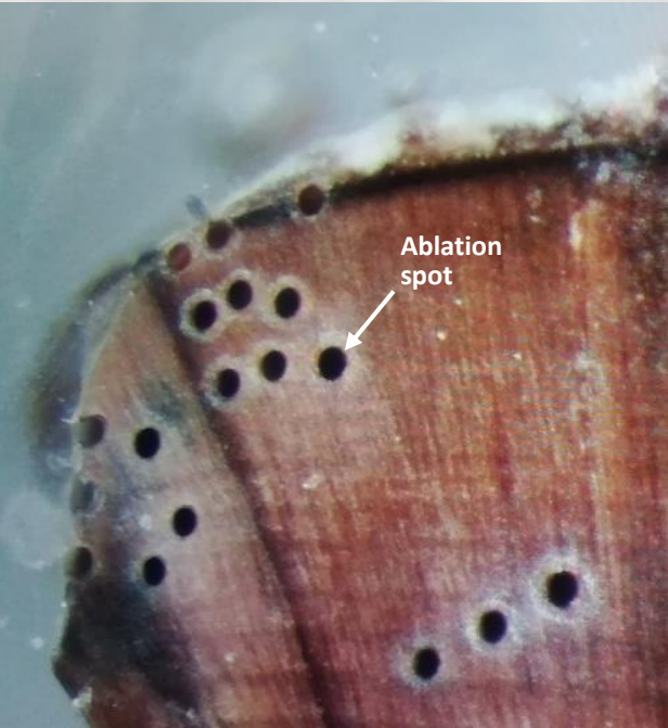
Polished teeth section used in the laser ablation ICP-MS analysis.
